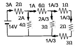
We now calculate the power dissipated in each resistor:
